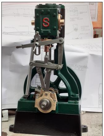
It has a 2" bore and stroke made in cast Iron.
